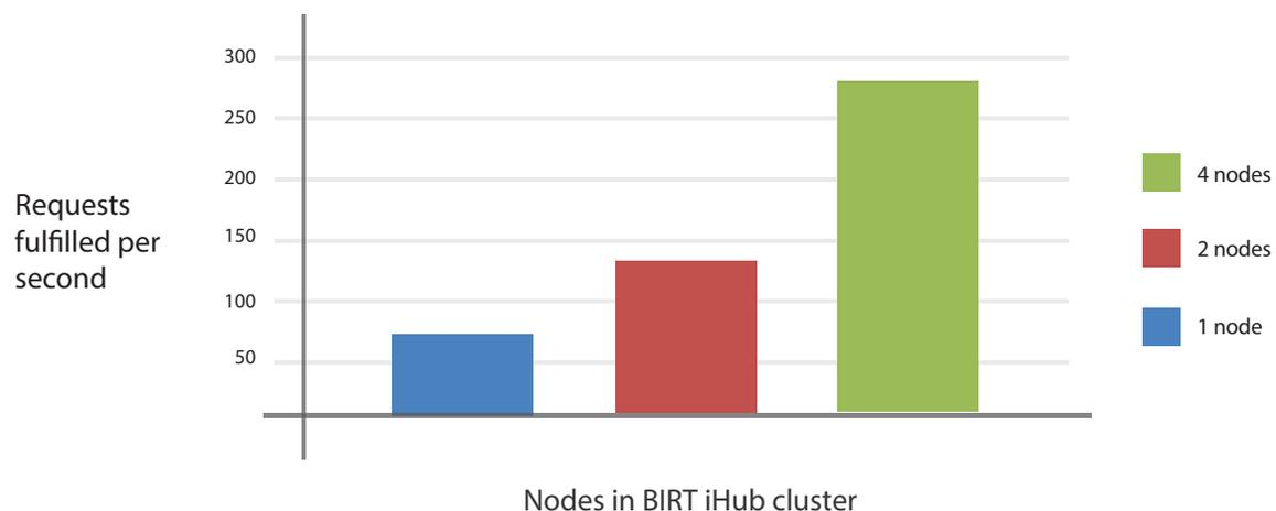
Figure 3: Linear scaling of the BIRT Online service, which handles on-demand viewing.
